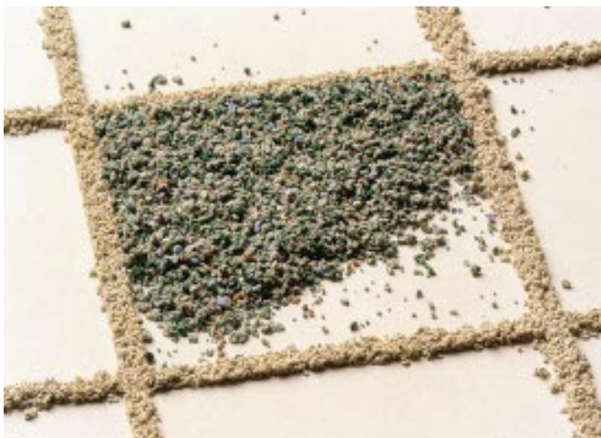
Figure 2. High-quality inlaid vinyl is made by heat-bonding colored vinyl chips to a carrier sheet. The products typically have a much thicker wear layer than lower-priced vinyls.
