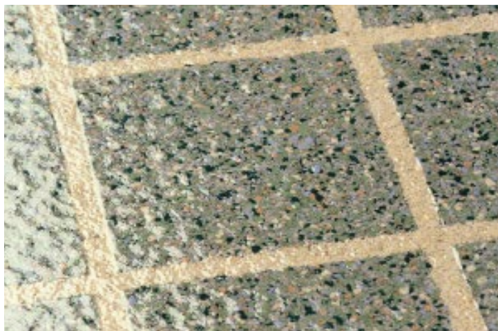
Figure 2. High-quality inlaid vinyl is made by heat-bonding colored vinyl chips to a carrier sheet. The products typically have a much thicker wear layer than lower-priced vinyls.
