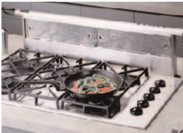
Figure 3. A downdraft vent's performance is enhanced by rising to meet the heat. This unit will rise 9½ inches above the cooktop to handle tall pots.
