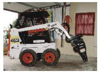
model in the loader line, with a 700-pound capacity and a 10-gpm hydraulic system that will power at least 20 different attachments, including a bucket, auger, trencher, grapple, utility forks, and the breaker shown here. With the narrowest tires available, it's under 35<sup>1</sup>/2 inches wide. Just imagine the possibilities, at a suggested list of \$12,500.
