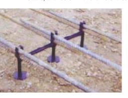
triple runs using #3, #4, or #5 rebar. The Model RC-6-2 is 6 inches wide. Model RC-12-3 is 12 inches wide; both are 3 inches high. These chairs are made of plastic, so they will not corrode, and they have a dual clamping feature that allows you to overlap the rebar by snapping the steel
