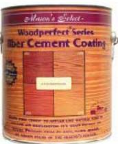
making the siding look like real wood, according to the manufacturer. The UV-resistant 100% acrylic latex coating protects the siding from water damage and mildew and dries to touch in one hour. Four factory-designed colors (mahogany, maple, redwood, and cedar) can be mixed to create other colors. Coverage is 175 to 275 square feet per gallon, depending on
