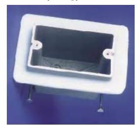
ceilings. The fiberglass-reinforced nonmetallic outlet boxes, available in a variety of shapes and sizes, use a polyurethane flange to form a vapor seal for greater energy efficiency.
