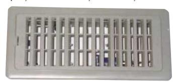
AZR (Automatic Zone Register). Instead of mounting midstream in the ductwork like most zone dampers, the AZR slips into an existing register opening, with no modifications to existing ducts. Run a plenum-rated 'stat wire back through the duct to a zone panel or stand-alone thermostat, and you're done. Sizes are currently limited to 10x4, 12x4, 10x6, and 12x6, with prices starting at around \$50.
