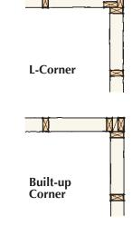
for supporting the building's vertical load and provide little significant benefit to improve a frame's racking resistance, which is provided by the nailed sheathing.
