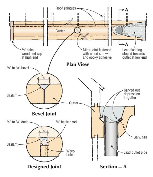
miter joint, fastened with screws and adhered with epoxy adhesive formulated especially for wood.
