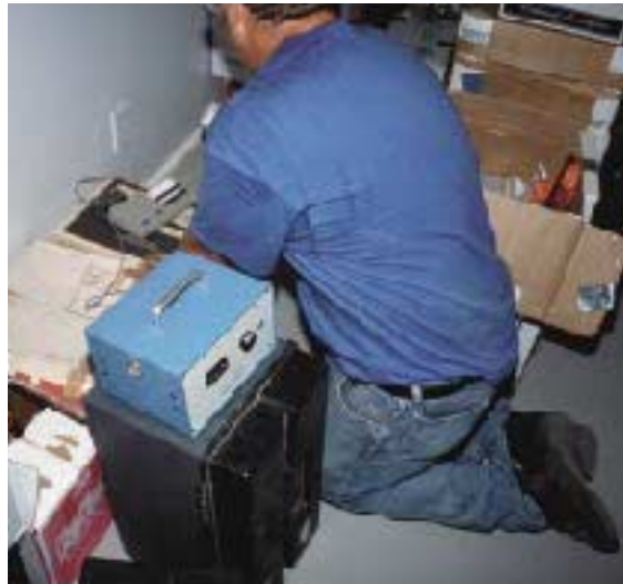
Figure 8. An electronic radon-monitoring device continually tests the amount of gas present. Once each hour, it prints out the current radon level as well as an average that factors in all previous readings.
