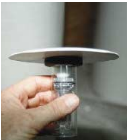
Figure 1. A special check valve is used to prevent the sub-slab ventilation system from sucking indoor air through the floor drain. It opens for drainage when weighted down by accumulated water, but when the drain is dry, a spring-loaded ball provides a seal that maintains negative pressure beneath the slab (left). Once the valve has been cemented in place (center), any visible cracks in the slab or foundation walls are repaired with a durable sealant (right).
