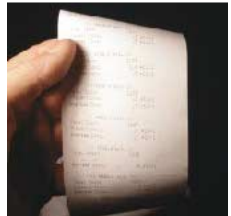
Figure 9. After four days of continuous testing with two separate monitors, the highest average recorded came out at .5 pCi/L — comfortably below the 4 pCi/L action level.
