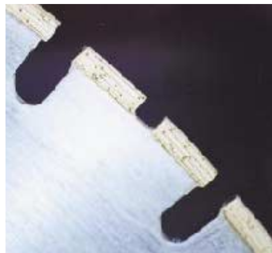
Figure 3. Various combinations of metal hardness and diamond friability produce industrial diamond saw teeth, called segments, suitable for different types of aggregate and concrete hardness. Blade design ensures that water is thrown into the cut by centrifugal force.
