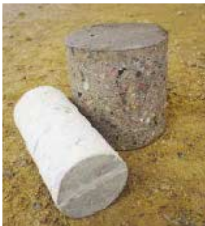
Figure 9. Concrete cores, 2 to 12 inches in diameter, are cut with a wet-sawing rig bolted or vacuum-mounted to the surface being cored. The resulting holes can accommodate water or sewer lines, wiring, or duct-work.
