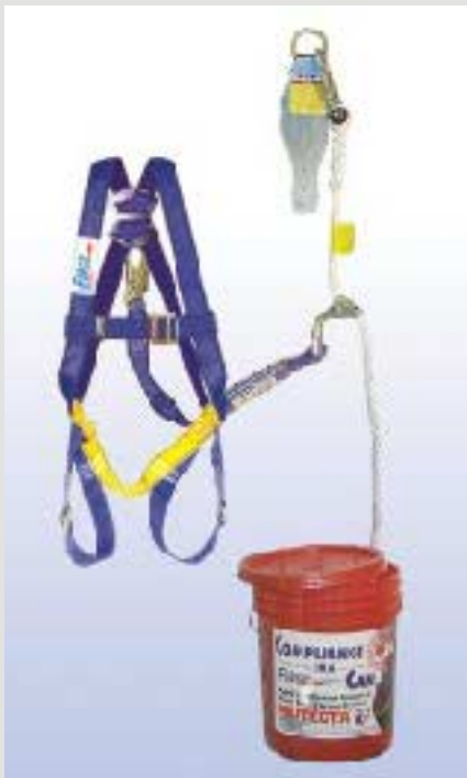
Figure 1. A Personal Fall Arrest System typically consists of an approved building anchor, a body harness, a lifeline, a connecting device, and a lanyard. Many manufacturers bundle the necessary components in a kit like the $163 Compliance in a Can from Protecta Corp. (left). A body belt may be used for restraint or positioning — to prevent a worker from approaching the edge of a flat or low-slope roof, for example — but must never be used where there's a chance that a vertical fall may occur (right).
