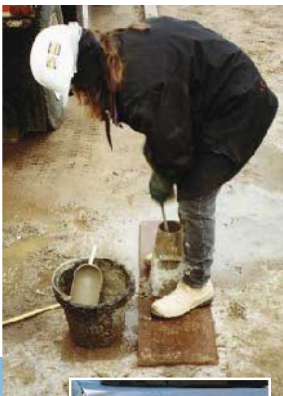
Figure 6. Although few residential contractors use them, slump tests ensure that the concrete coming out of the truck is not too wet (right). If better flow is needed, add a superplasticizer (below).
