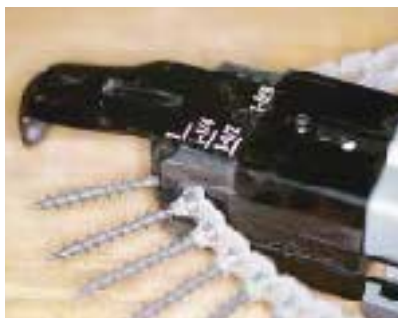
The Senco DS200-14v shoots screws from 1 to 2 inches long. According to the author, it has excellent balance and precise depth-of-drive adjustment.
