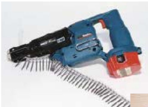
The Makita 6831DWA drives screws up to 1 5 / 8 inches long. It comes standard with one battery.
