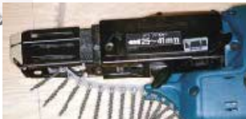
The Makita 6831DWA drives screws up to 1 5 / 8 inches long. It comes standard with one battery.
