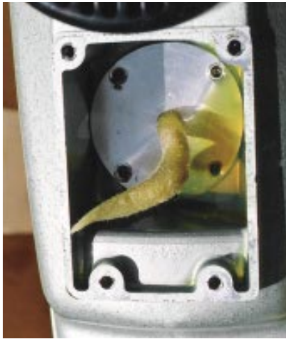
Figure 3. An oil bath with a wick provides lubrication for the Hitachi and must be topped off occasionally.
