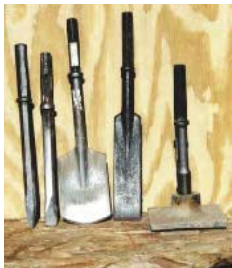
Figure 2. Along with the usual bull and chisel points, you can get a clay spade, a digging chisel, a tamper, and many other accessories.
