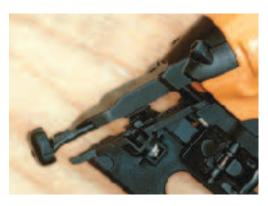
The front of the Bostitch gun is particularly sleek because jams are cleared by popping the magazine back from the nose.
