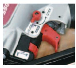
Max's NF550 features both a trigger lock and an anti-double-fire mechanism.
