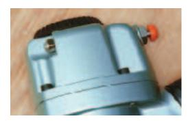
A built-in air gun on the Hitachi nailer makes it possible to clear dust from the work without using a separate air nozzle.
