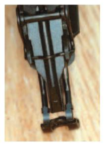
DeWalt's tip protector is bonded to the contact element and doesn't block your view of the work.
