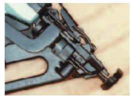
It's easy to gauge depth-of-drive on the Hitachi nailer because the adjuster wheel is indexed to a scale.
