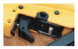
DeWalt's depth-of-drive is easily adjusted by sliding a button under the trigger.
