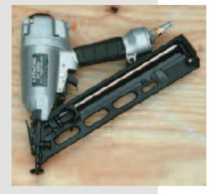
plenty of power and features, like an in-line magazine, a well-padded grip, and no-tools jam clearing. Unlike that of most guns, the depth-of-drive is indexed to a scale. The most unusual thing about this tool is the blow gun, which consists of a small nozzle and trigger button built into the piston housing. It may be a bit of a gimmick, but I love this feature because it means I can blast dust and debris out of the way without having to connect a separate blow gun.
