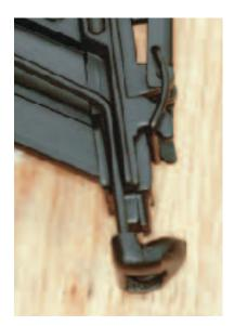
The contoured tip on the Porter-Cable gun makes it easier to nail from an angle.
