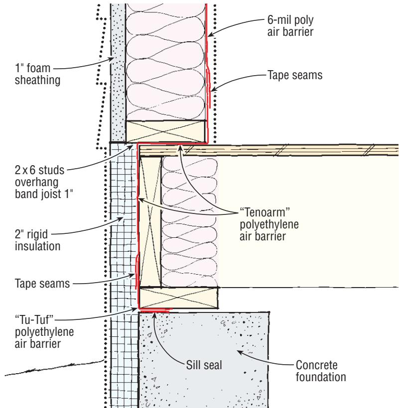
**Figure 3.** The key to the author's airtight shells is the continuous vapor barrier, which starts beneath the mudsill. Every seam is taped or sealed with acoustical sealant.
