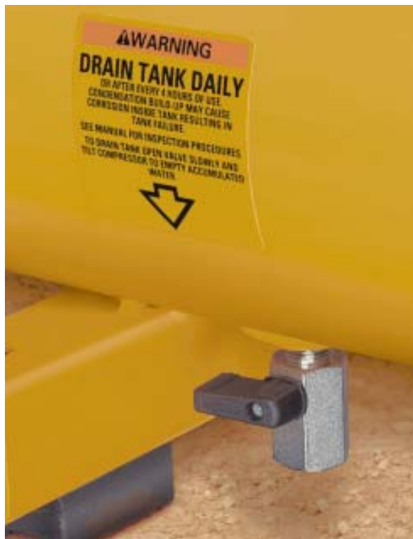
Figure 5. Draining water from your compressor daily will go a long way toward making tools and compressor last longer. Rusty tanks can force particles into pneumatic tools, damaging O-rings and soft aluminum parts, and a badly rusted tank could explode under pressure.
