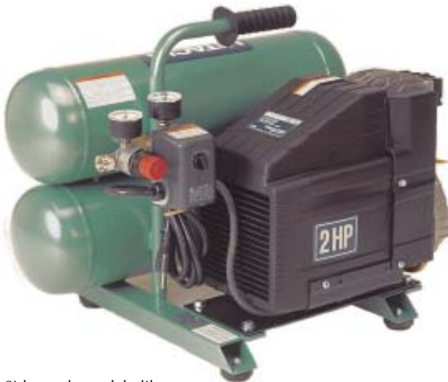
Figure 2. Side-stack models like these from Hitachi and Bostitch perform better than pancake designs. Their smaller size means that they won't be able to keep up with a framing crew, but their compact size, low center of gravity, and small amperage draw make them well suited for remodeling.
