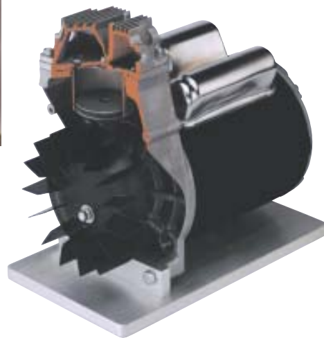
Figure 4. On an oil-lube model (above), the piston dips into a shallow oil bath. Setting up one of these on a steep pitch, like a roof, spells disaster. Super-slick oil-free models, like the one at right, require no oil but may not last as long.
