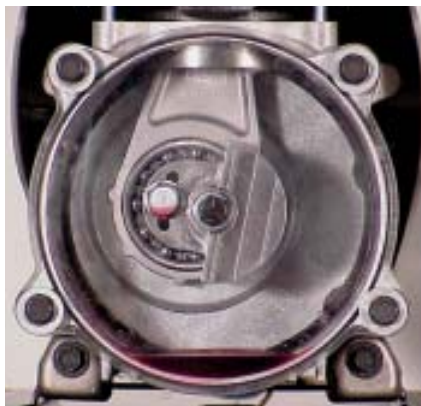
Figure 4. On an oil-lube model (above), the piston dips into a shallow oil bath. Setting up one of these on a steep pitch, like a roof, spells disaster. Super-slick oil-free models, like the one at right, require no oil but may not last as long.
