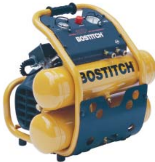
Figure 2. Side-stack models like these from Hitachi and Bostitch perform better than pancake designs. Their smaller size means that they won't be able to keep up with a framing crew, but their compact size, low center of gravity, and small amperage draw make them well suited for remodeling.
