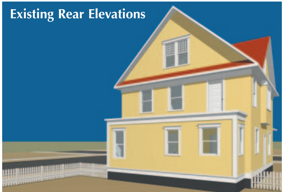
Figure 2. The blank, uninviting rear of the house is utterly disconnected from the back yard. Although most foursquare roofs were hipped — often with a central dormer in front — this one features a cross-gable roof instead. The second floor “rug-shaker door” opening onto the flat-roofed extension was considered quite a housekeeping convenience in its day.
