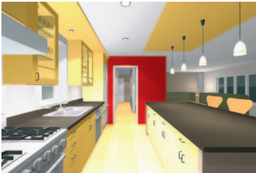
Figure 2. The remodeled kitchen, now open to the living and dining rooms and focused on an island, shows four different lighting strategies that can be used simultaneously or independently, which makes the kitchen more flexible.
