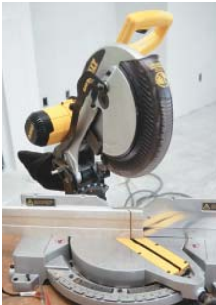
Figure 5. When mitering baseboard for an inside corner at each end, the left miter is cut first, with the saw tilted right and the material right side up (left). The material is slid to the left and marked to length on the back-bottom corner. To make the right-hand cut, the baseboard is turned upside down on the fence, leaving the mark facing up and clearly visible (right).
