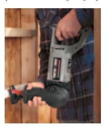
fortable. The front gear housing allows the blade to rotate 360 degrees, and another pivot, just in front of the motor housing, swivels through a 180-degree range of motion. With the back pivot perpendicular to the saw body, the Tiger Claw measures a mere 81/2 inches long. The new saw should be a real help to mechanical installers
