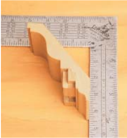
Figure 1. With the top of the square as the ceiling, the rise of the crown molding is measured to the bottom of the crown.
