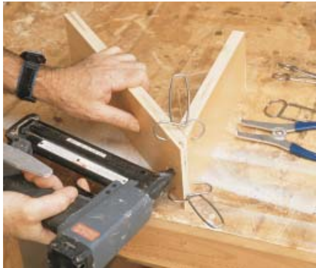
Figure 19. The author used two scraps of \frac{3}{4} -inch plywood about a foot long by 4 inches wide for the accessory fence, both cut with 45-degree miters on the ends (left). The fence is attached to a \frac{3}{8} -inch plywood base, which hangs about 4 inches past the fence to provide a base for moldings (center). For safety and tight joinery, be sure to clamp the fence to the saw and the material to the fence before cutting (below).
