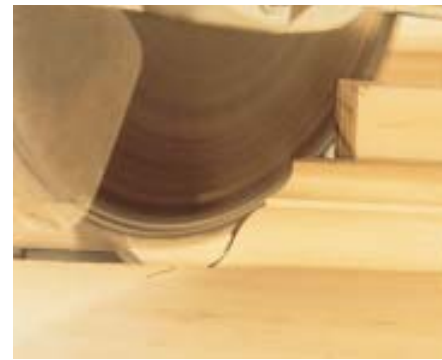
Figure 4. The long point of an inside corner is always against the wall or fence (left). The short point of an outside corner is always against the wall or fence (right).
