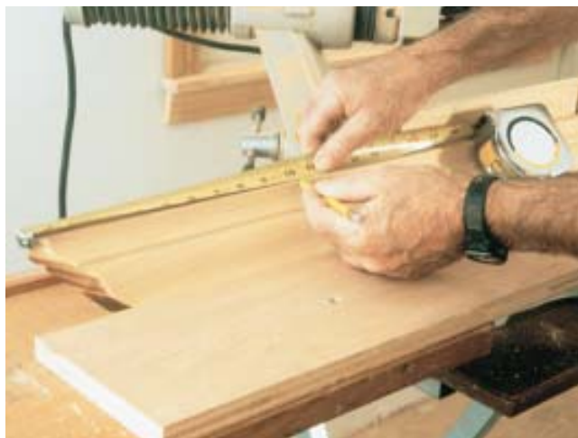
Figure 5. Measure an inside corner by hooking the tape over the long point.
