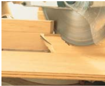
Figure 4. The long point of an inside corner is always against the wall or fence (left). The short point of an outside corner is always against the wall or fence (right).
