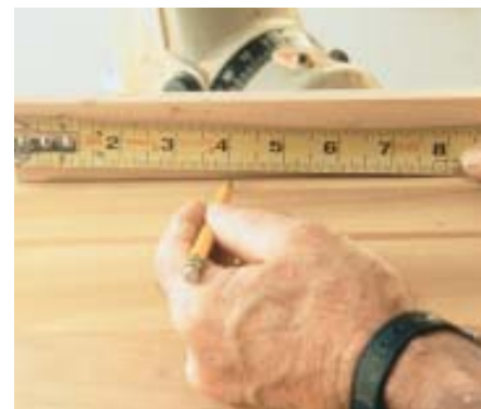
Figure 6. Measure an outside corner by aligning the short point with the edge of the saw fence and hooking the tape over the fence.
