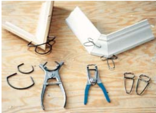
Figure 16. For preassembling crown, casing, and panel moldings, miter clamps are the secret. Ulmia clamps are on the left, Collins clamps on the right.
