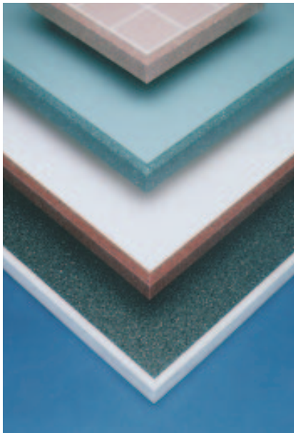
Figure 3. Solid-surface edging offers a durable, attractive treatment with near-foolproof application and custom corner profile capability. This option is adaptable to most countertop materials, including high-pressure laminate.
