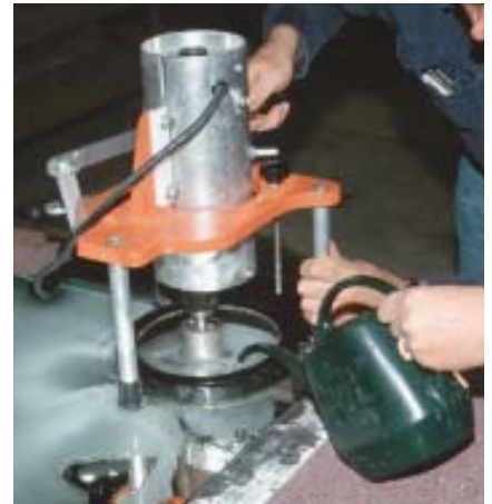
Figure 3. A proprietary tripod drill press uses diamond abrasive bits to cut circular openings in mirror glass.
