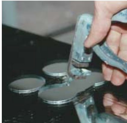
Figure 4. To create a rectangular box opening, the author drills multiple holes, then finishes the job with a scoring tool and a nibbler.
