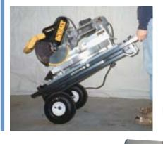
Moving the HTC while it's folded is easy. All its parts fit into a single unit, and air-filled tires cushion the ride. The HTC has useful roller and bar-type supports. The position of the tires makes the stand hard to move while it's set up: It requires another person to help, or you'll have to break it down, which takes a few minutes. The adjustable middle support can be raised slightly to function as a stop (below left).
