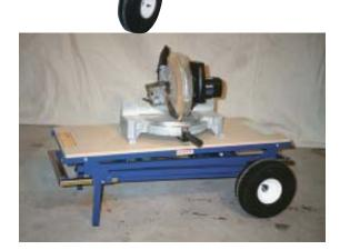
The MS2000 has an impressive 154-inch capacity when set up but folds to wheelbarrow size. The <sup>1</sup>/2-inch tubular stock on its extension tables seems a little flimsy and might bend if subjected to a heavy load.
