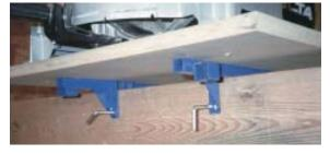
The Trojan Workcenter's no-frills design relies on a 2x6 to support the saw base. It clamps securely and allows the user to vary the length of the stand as needed, depending on the length of the 2x6 selected.
