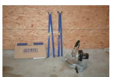
Although the Workcenter breaks down into a number of separate units, all the components (excluding the saw) will fit neatly behind the seat of a pickup. When the saw stand is not in use, the folding sawhorse legs and rollers can be used for other tasks.
