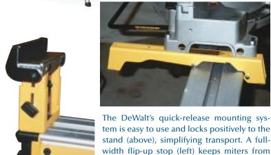
slipping past, but the stand's compact design limits the maximum stop setting to 8 feet.
