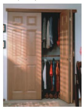
have to fabricate out of a scrap of pine? The *Johnson 1700 Folding Door Hardware Kit* promises to make the bifold installer's life easier. For one thing, the top track hangs the entire weight of the door on surface-mounted brackets — no more drilling pivots and guides into the door. The rugged track is easy to mount and adjust, and, best of all, the bottom bracket mounts to the doorjamb, not the floor. The 1700 costs \$15 to \$25 per kit, depending on door size.
