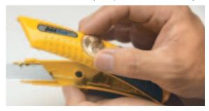
Cutter. The QuickBlade has a thumbwheel release dial where the screw usually is, a blade carrier that can't fall out, and a hinge at the back of the knife to keep the two halves together while you're changing blades. It retails for around \$7.
