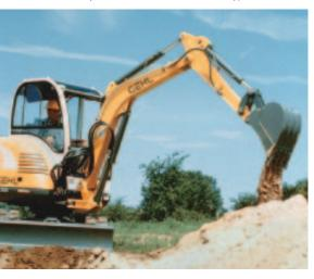
horsepower model that has a digging depth of 14 feet 9 inches. Standard features include auxiliary hydraulics, two-speed drive train, dozer blade, and a wide variety of attachments. The cab and boom swing independently to weasel into tight places. Pricing starts
