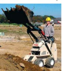
inches wide — allows users to get into spaces only a shovel and wheelbarrow could go before. The Eagle has more than 40 attachments, and the universal faceplate allows the use of accessories from other manufacturers. With a 25-horse-power engine and full-flow hydraulics, it has enough power to run multiple hydraulic func-
