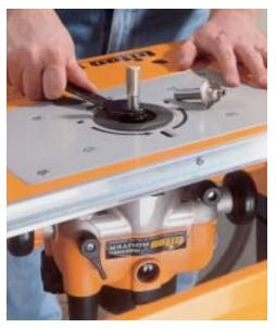
and can bring the <sup>1</sup>/<sub>2</sub>-inch collet proud of the base, making adjustments and bit changes easier than with other routers. The depth adjustment knob can be disen-
