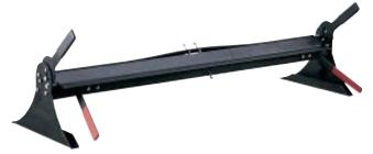
job-site metal-bending tasks. It can handle sheet metal up to 22-gauge and 4 feet wide. Any length is possible because the tool doesn't have a fixed throat. Extra wide feet provide good stability, and a heavy-duty cam-over clamping mechanism holds the metal securely. Companion legs for the Mini Brake are sold separately. With a street price of under \$300, the Mini probably won't brake the bank.
