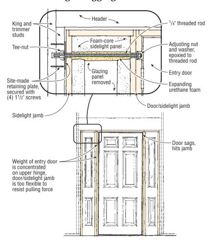
Threaded rod, drilled clear through a flanking sidelight into the framing just high enough to clear the glazing, counters the weight of an entry door at the topmost hinge and prevents it from sagging. A site-made steel retaining plate prevents the tee-nut connector from pulling out of the framing under tension. The adjusting nut is recessed in the hinge jamb, just above the hinge.
