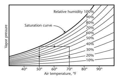
A psychrometric chart provides the dewpoint for any given air temperature and relative humidity. Say you have a relative humidity of 50% at 70°F. On the horizontal scale, locate the air temperature and move up to the curve that represents 50% relative humidity. Then move left to the saturation curve and down to find the dewpoint — 50°F in this case.
