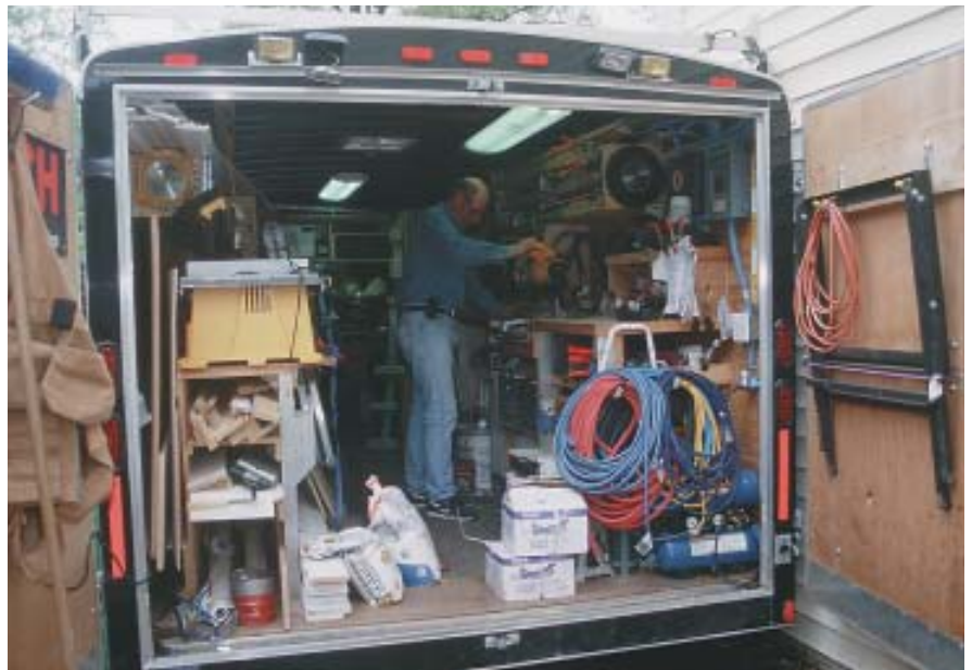
Figure 1. A power miter saw and a swing-up 10-foot sheet-metal brake are always ready on their respective benches. A built-in shop-vac dust collector under the bench keeps the cutting table clear of sawdust.
