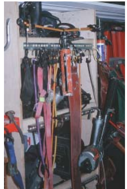
Figure 2. Frequently used tools hang from quick-release carabiner clips for easy access and return, and to prevent spilling during travel. Bungee cords and raised shelf lips help keep stored items in place.
