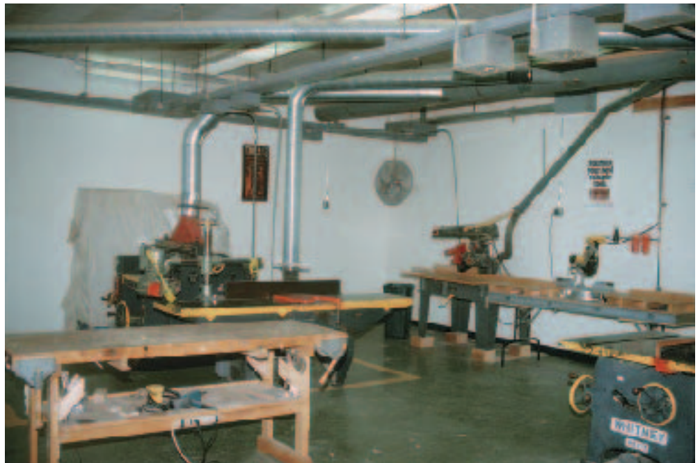
Figure 1. This woodworking shop created noise levels equivalent to the sound of a jet plane taking off. The noise was like a loud stereo in the adjacent office. The solution was to shrink the shop, adding a sound-dampening wall and a buffering hallway (below).
