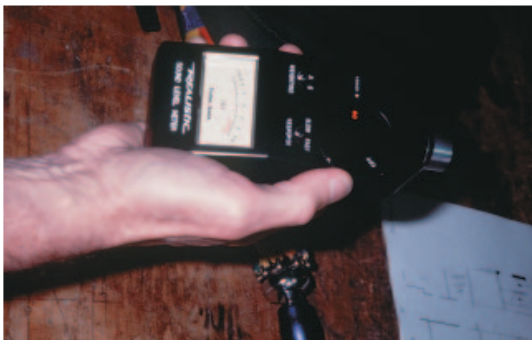
Figure 2. Using a hand-held sound meter, the authors measured the sound levels of the machinery in use.
