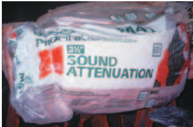
Figure 5. Sound-attenuation batts sized specifically for steel studs can improve partition STC ratings by as much as 10 dB.
