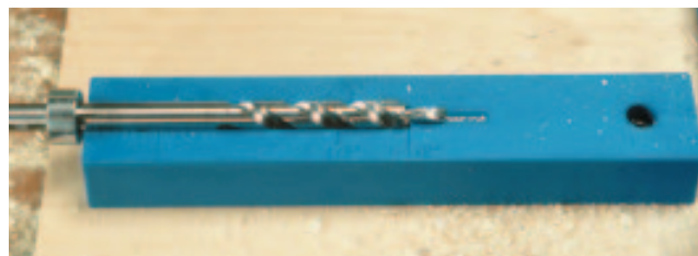
Figure 2. The jig's support wings include a handy guide for setting the stop collar on the drill bit.
