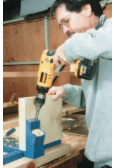
Figure 1. Mounted on a piece of 2x12 for greater stability, the Kreg jig makes quick work of pocket-hole joints.
