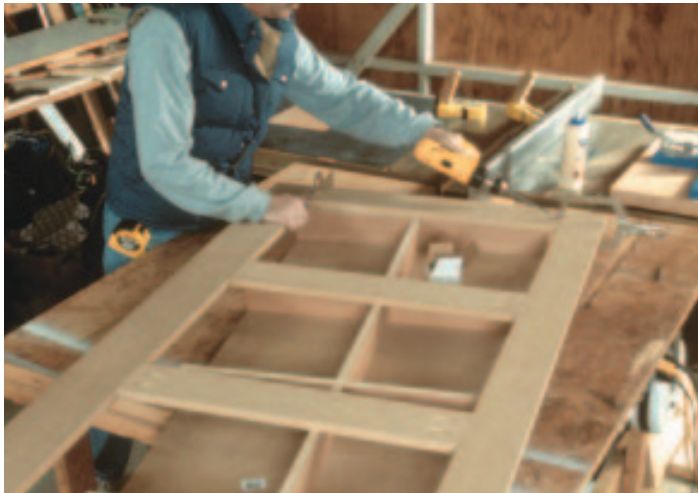
Figure 4. A simple plywood work grid makes it easy to manipulate face frames for making joints and glue cleanup (left). The vise-grip clamp holds joints secure for screwing (right).
