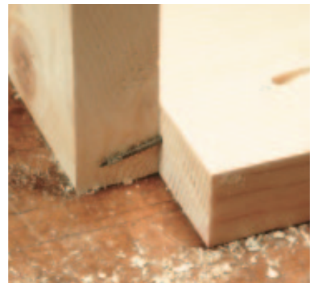
Figure 3. The Kreg jig can make joints in material from 1/2 inch to 1 1/2 inches thick.
