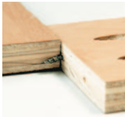
Figure 3. The Kreg jig can make joints in material from 1/2 inch to 1 1/2 inches thick.
