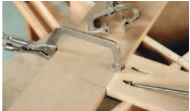
Figure 4. A simple plywood work grid makes it easy to manipulate face frames for making joints and glue cleanup (left). The vise-grip clamp holds joints secure for screwing (right).
