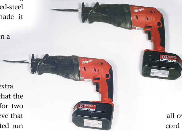
Figure 2. The Hatchet's battery can be spun around to keep its ample size out of your way. The 2.4-amp-hour pack charges in a little under an hour and powers the tool for about 15 minutes of continuous, heavy-duty cutting.
