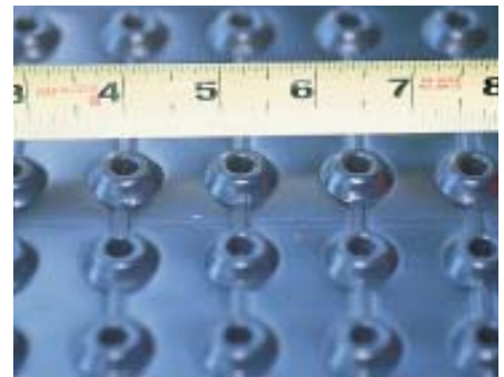
Figure 6. Air-gap membranes, like Cosella Dörken's Delta-MS (left) and System Platon (above), have raised dimples that allow any water that gets past the membrane to fall to the footing drain.
