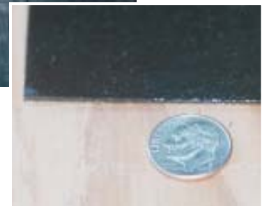
Figure 4. Sheet membranes, like Grace's Bituthene, shown here, apply like peel-and-stick eaves membranes. Inside corners are first coped with proprietary sealants (above left), then the membrane is pressed into place (above right). Most sheet membranes are around 60 mils thick, or about one and a half times as thick as a dime (right).
