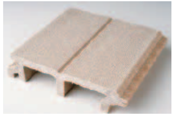
Figure 2. Hollow products, like TimberTech, are lighter in weight than solid composites. Installers generally use skirting or trim pieces to hide the cut ends.
