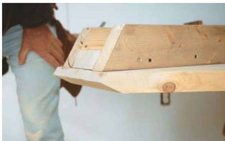
Align and fasten the jig block along the beveled plumb cut (top). With the circular saw set to cut at 90 degrees, cut down the center of the bevel face using the jig as a base for the saw (middle). Above, the finished 62-degree cut.
