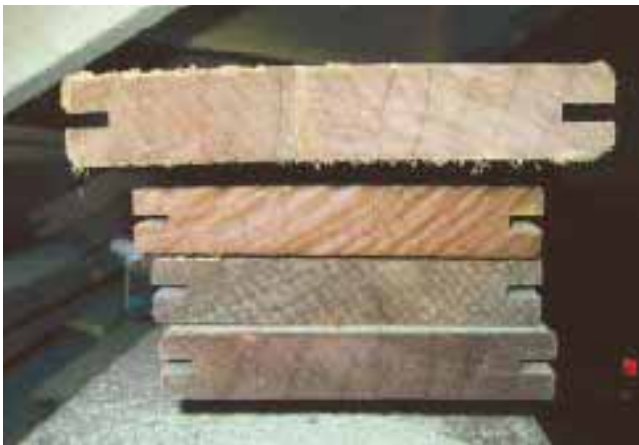
Figure 9. Tropical hardwood decking is fastened with the Eb-Ty connector system, which uses a slot-mounted plastic biscuit. Rather than cutting individual slots with a biscuit jointer, the author increases productivity by ordering deck boards with premilled grooves.
