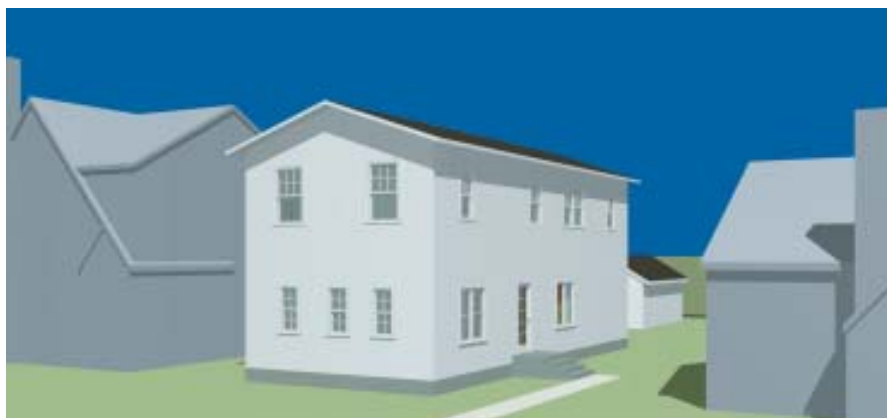
Figure 2. Extending the first-floor walls and adding a standard 4/12-pitch roof truss with an 8-foot flat ceiling provide the needed space at the lowest possible cost, but the result is visually awkward and out of place.
