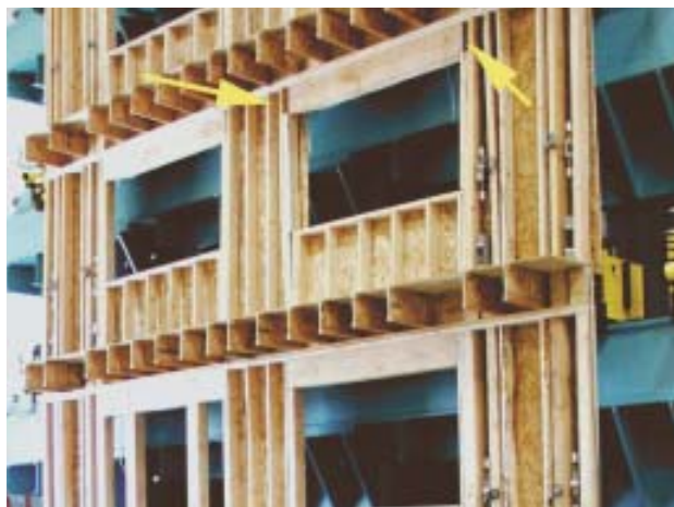
A three-story wall section is mounted on a shake table at Simpson Strong-Tie's Stockton, Calif., test facility (above). After a good shaking (right), it shows extensive damage, including cracked plates and buckled sheathing. The arrows indicate where the headers above the second-floor opening have separated from the king studs.
