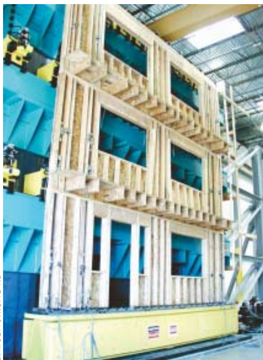
A three-story wall section is mounted on a shake table at Simpson Strong-Tie's Stockton, Calif., test facility (above). After a good shaking (right), it shows extensive damage, including cracked plates and buckled sheathing. The arrows indicate where the headers above the second-floor opening have separated from the king studs.
