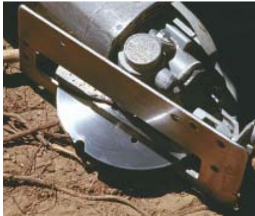
Figure 1. The author's crew gang-cuts as many as seven pieces at a time using a wormdrive saw (above). In contrast with a regular carbide blade, which would be dull after a single day of cutting, this dedicated fiber-cement blade from James Hardie has cut the siding for five 2,500-square-foot houses (right).
