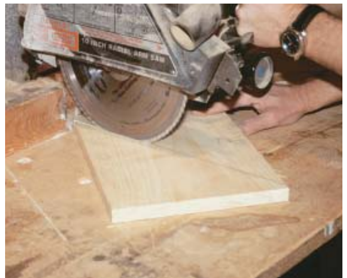
Figure 1. A pitch block is a simple gauge that's useful for determining post and rail height adjustments on offset newels. It's easily made by marking the diagonal between tread and riser on a square-cut lumber scrap (left), then cutting it to the line with a radial arm saw (right).
