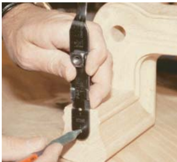
Figure 6. A built-in gauge on the proprietary rail-bolt wrench provides necessary drilling centers for bolt and access holes. Drilling the access hole before the bolt hole prevents the access-hole bit from wandering when the lead spur intersects the bolt hole.
