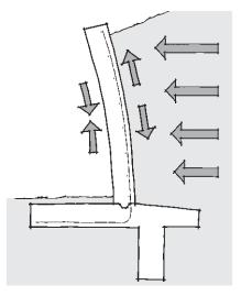
Think of the retaining wall like a vertical cantilever beam. When the soil pushes against the wall, it wants to deflect the way a beam would. It stretches on the soil side and compresses on the open face.
