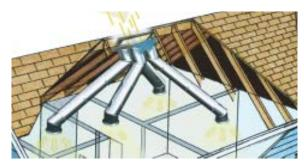
tration, installation should be faster and less expensive than for individual tubes. The Spyder can accommodate both 10-and 14-inch light tubes; add-on light kits are also available. A double unit with two 10-inch tubes starts at \$250.
