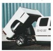
the labor saver you've been looking for. The Load Hog mounts invisibly under the bed and converts a standard full-size pickup truck into a pneumatically controlled dump truck, without changing its appearance. With a capacity of 4,500 pounds, it can unload a full bed of gravel, debris,
