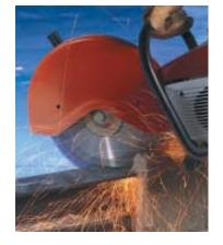
to the manufacturer, the blade, which is available in 7-, 12-, and 14-inch sizes, cuts through reinforced concrete without damaging the blade, allowing demolition of mixed materials without time-wasting blade changes. Prices for the 7<sup>1</sup>/4-inch blades start at \$89, 12-inch blades at \$129, and 14-inch blades at \$159.
