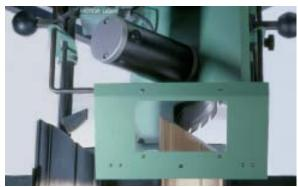
and can accommodate molding up to  $1^{1}/4$  inches thick and  $7^{1/2}$  inches wide. The 65-pound machine folds for transport. The price is \$1,895. Copemaster, 800/630-1104, www.copemaster.com.
