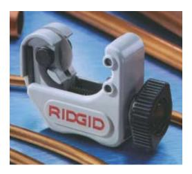
around the tubing until it cuts through. Close quarters require a mini cutter, a tiny version of the same tool. The tradeoff is an uncomfortably small knob for adjusting pipe size and tensioning the wheel as it cuts. Ridgid's Self-Acting Midget Cutter has a spring-loaded cutting wheel, so you don't have to keep turning a small knob as you cut through the pipe. The cutter works on copper, brass, and aluminum tubing from  $^{3}/_{16}$  inch to  $^{15}/_{16}$  inch. It lists for \$16.50.
