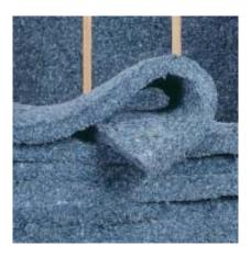
is made largely from denim scraps, so handling and installing the product requires no protective equipment or other special measures. According to the manufacturer, the borate-treated product performs better than fiberglass in extreme cold, is not as attractive to rodents and insects, and has excellent fire resistance (class 1). The 3<sup>1</sup>/2-inch, R-13 product runs about 50¢ per square foot, and the 5<sup>1</sup>/2-inch, R-19 runs about 70¢ per square foot.
