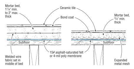
For thick mortar bed installations over wood floors (left), ANSI specs call for wire fabric reinforcing and a cleavage membrane between the subfloor and the mortar. For thin mortar beds (right), use expanded metal lath nailed or stapled to the subfloor.
