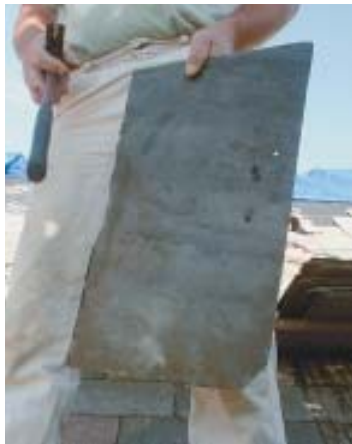
Figure 2. Sound slates make a crisp ringing sound when struck with a hammer. This piece, salvaged from an old Vermont barn, could provide another hundred years of service on a roof.
