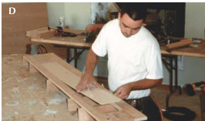
Figure 2. Pocket screws make for tight joints between rails and stiles (A) and allow the frames to be handled while the glue is still wet. In a quick operation, a carpenter rabbets the frame (B), then installs the panel with glue and staples (C, D, E). The panels were cut 1/8 inch smaller than the overall width to allow for seasonal movement.
