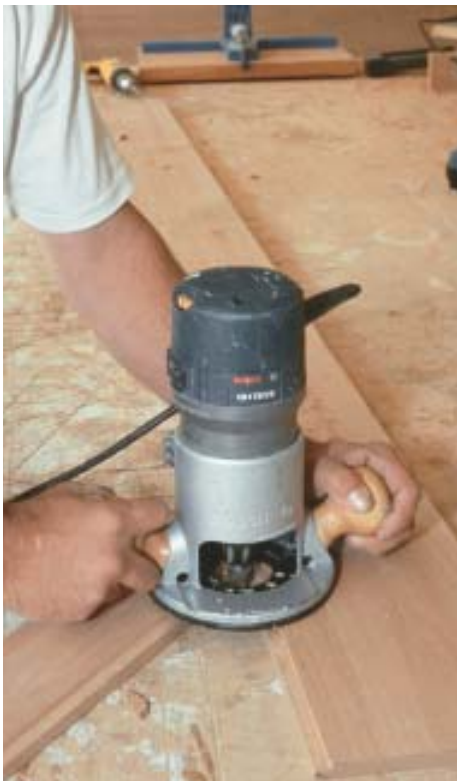
Figure 5. The routed inside-corner rabbets on angled panels (above) were finished by hand (right).
