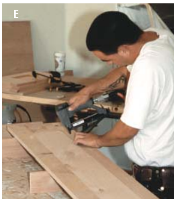
Figure 2. Pocket screws make for tight joints between rails and stiles (A) and allow the frames to be handled while the glue is still wet. In a quick operation, a carpenter rabbets the frame (B), then installs the panel with glue and staples (C, D, E). The panels were cut 1/8 inch smaller than the overall width to allow for seasonal movement.
