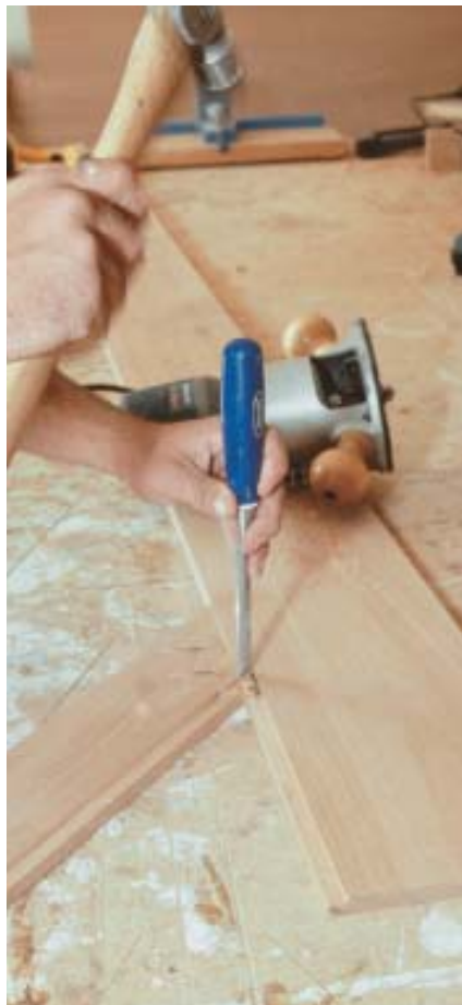
Figure 5. The routed inside-corner rabbets on angled panels (above) were finished by hand (right).
