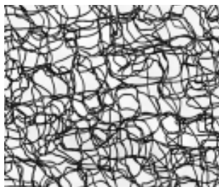
Figure 4. Tangled open-weave fabrics made from heavy plastic strands (right) provide a tough anchorage for plants to resist stormwater erosion and trap silt. Wrapping heavy fabrics around soil on an exposed river or lake bank can hold the bank in place and help plants stay anchored (below).
